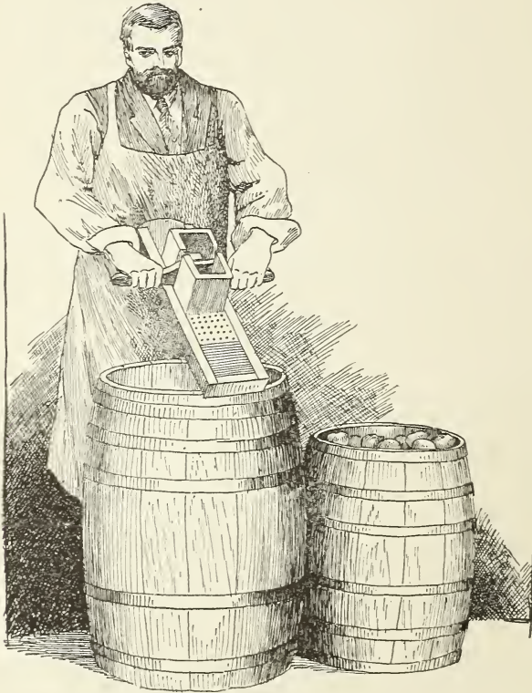
FIG. 3.—Primitive apple grater in use in Germany.
